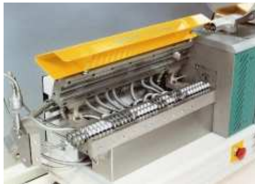
Figure B-7 Extrudeuse bi-vis co-rotative Thermo Prism PTW-16 de Thermo Haake
