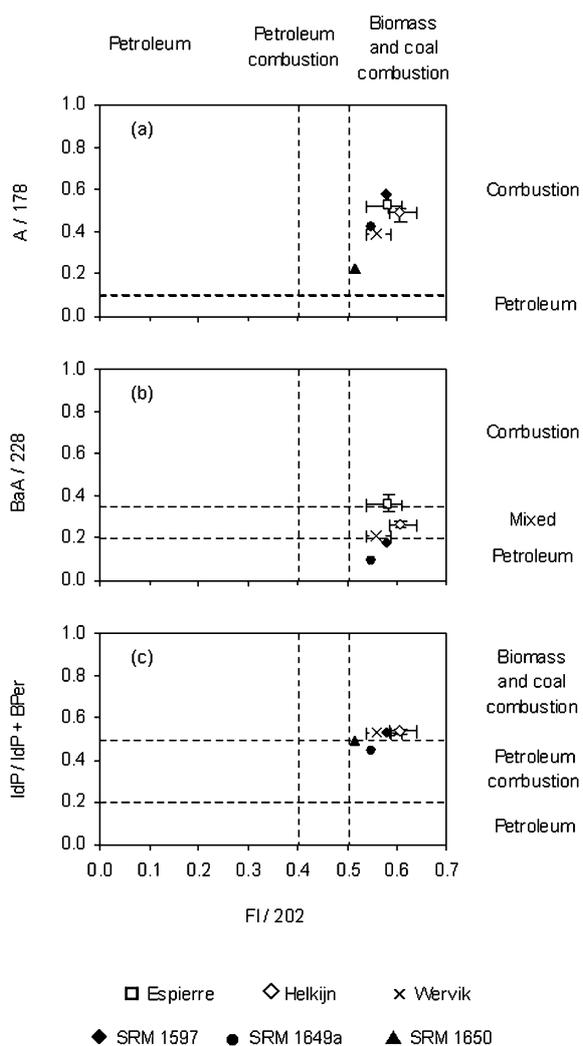
**Fig. 4** PAH isomer pair ratios of reference materials and of sediments for the three sites (minimum and maximum values). The ratio FI/202 is plotted against the ratios (a) A/178, (b) BaA/228 and (c) IdP/IdP + BPer. The graphic representation is based on Oros & Ross.<sup>37</sup>
