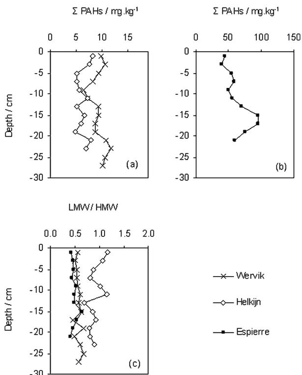
**Fig. 3** Sedimentary depth profiles of the total PAH concentrations ( $\Sigma$  PAHs) in  $\text{mg kg}^{-1}$  ((a)Wervik and Helkijn cores and (b) Espierre core) and (c) the ratio of low molecular weight PAHs on high molecular weight PAHs (LMW/HMW) in the three sediment cores.
