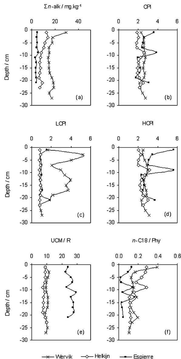
**Fig. 2** Sedimentary depth profiles in the three sediment cores of (a) the total *n*-alkane concentrations ( $\Sigma n$ -alk) in mg kg<sup>-1</sup> and of the aliphatic indexes: (b) CPI (carbon preference index), (c) LCPI (low range carbon preference index), (d) HCPI (high range carbon preference index), (e) UCM/R (unresolved complex mixture/resolved compounds) and (f) *n*-C18/Phy (*n*-C18/phytane).
