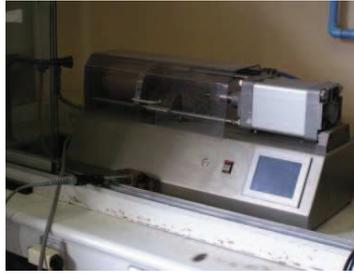
Figure 23: Micro-presse à injecter DSM Research Explorer
