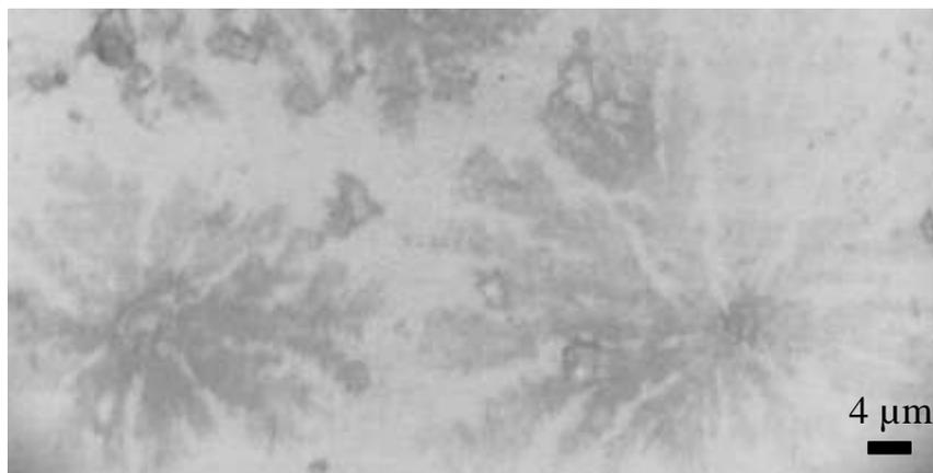
**Fig. 5.4** 100x optical image of  $\text{NaC}_{18:1}$  thin deposits formed after drying of a CMC aqueous solution deposited on mica(001).
