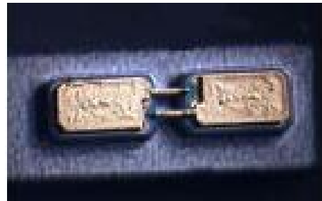
Figure 7 Diode Schottky planaire AsGa
