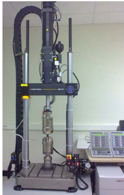
Figure 4.2.2. Machine de fatigue en traction-torsion Instron-8874.
