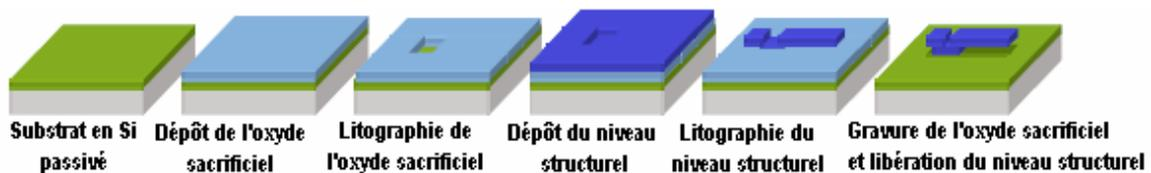
Figure 61. Micro-usinage de surface [Delauche 2003]
