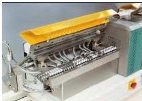
**Figure B-5** : Extrudeuse bi-vis co-rotative Thermo Prism PTW-16 de Thermo Haake
