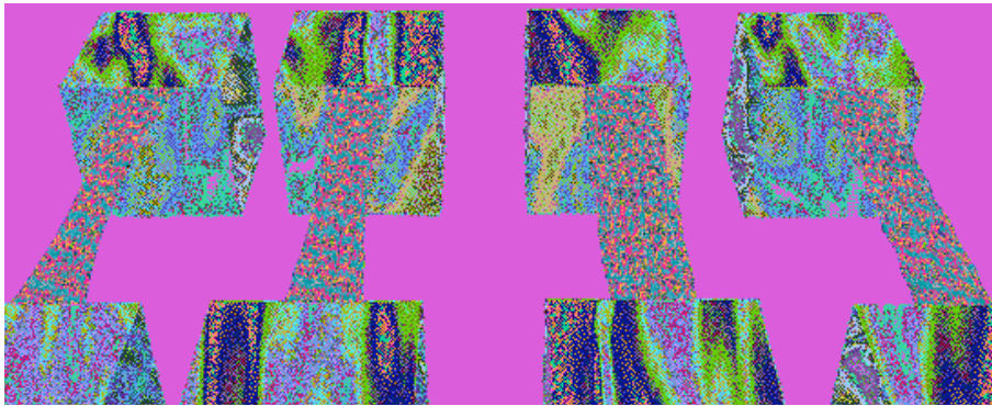
Figure 7.3: A 400% stretched fabric square with various Poisson's ratio. Image courtesy of Volino and Magnenat-Thalmann (1997) .
