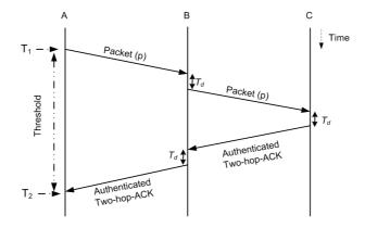
T<sub>d</sub>: ( Processing + queuing ) delay at nodes B and C
