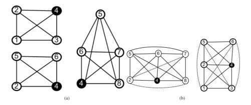
FIGURE 6.7: The set of maximal cliques. (a)  $R_{cs} = R_{cs1}$ , 3 maximal cliques whose sizes are 4, 4 and 5 respectively; (b)  $R_{cs} = R_{cs2}$ , 2 maximal cliques of 6 vertices each. Note that the dashed edges represent the new links created due to increase in  $R_{cs}$  from  $R_{cs1}$  to  $R_{cs2}$
