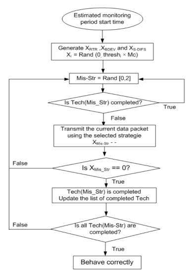
FIGURE 5.2: The switching scheme used by the adaptive cheater to switch over the cheating strategies
