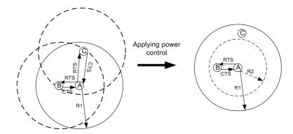
FIGURE 4.14: Impact of power control employment on the transmission range of node A, A's transmission range reduces from R1 to R2
