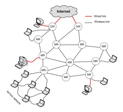
FIGURE 2.2: Wireless Mesh Network Architecture
