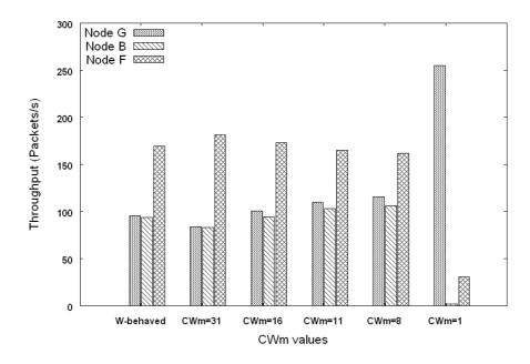
FIGURE 6.8: Propagation of greedy behavior's impact according to  $CW_m$  variation in MANETs, measured in terms of the acquired throughput.
