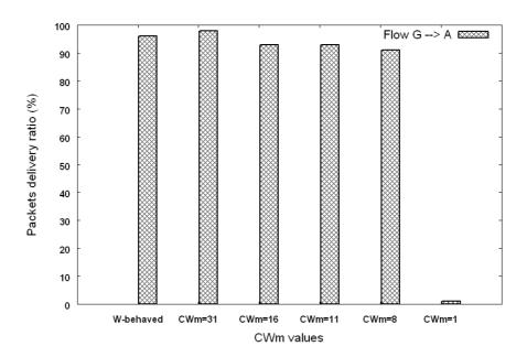
FIGURE 6.10: Variation of the packet delivery ratio of the greedy node's flow versus the chosen  $CW_m$  value
