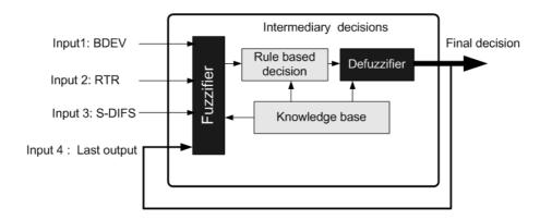
FIGURE 5.7: The main components of FLSAC
