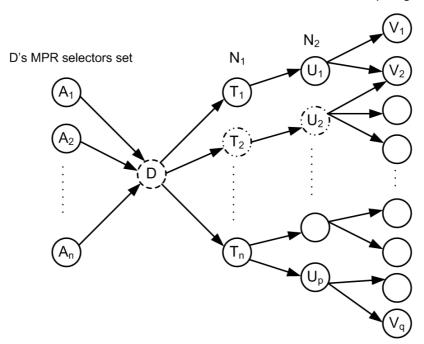
FIGURE 4.2: Colluding black hole attack model
