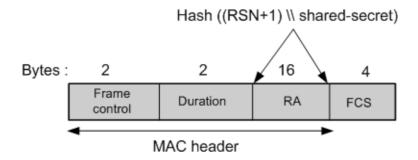
FIGURE 4.17: The format of CTS+ frame (24 bytes)
