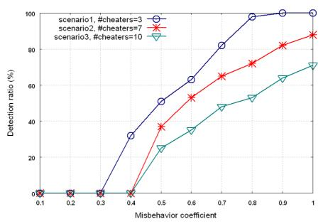
(a) Detection ratio versus misbehavior coefficient
