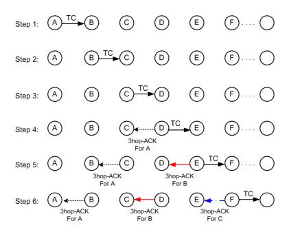
FIGURE 4.8: The  $3hop\_ACK$  scheme functioning
