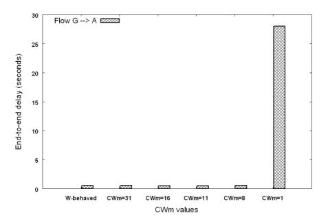
FIGURE 6.9: End-to-end delay of the greedy node's flow versus  ${\cal CW}_m$  size.
