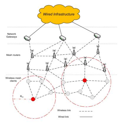
FIGURE 5.1: Wireless Mesh Networks model
