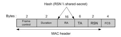
FIGURE 4.16: The format of RTS+ frame (32 bytes)
