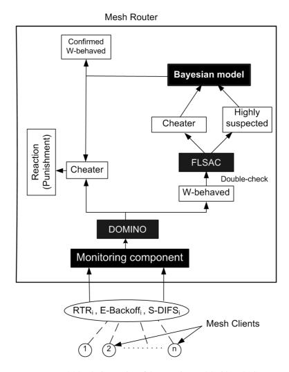
FIGURE 5.14: The integration of the Bayesian model with FLSAC
