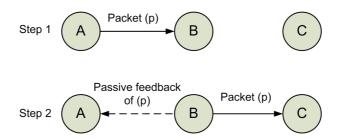
FIGURE 3.9: The principle of passive feedback
