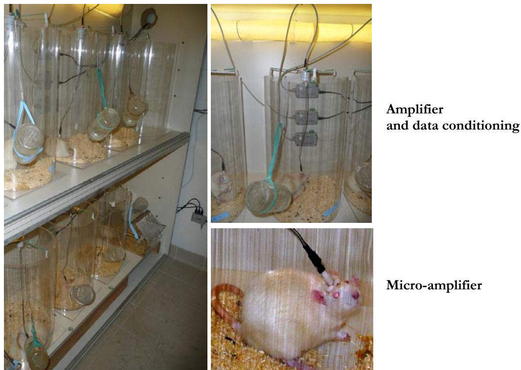
FIG. 30: Pictures of sleep recording room and detail of rotating swivel.
