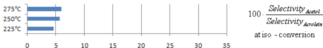
Figure 5-9: Selectivity ratio for 20 wt.% silicotungstic acid on CARiACT Q-10 at different reaction temperatures
