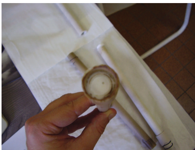
Fig. 4.6 Picture of a membrane sealed with pyrex glass.
