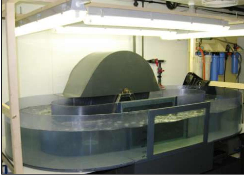
Fig. 14. Photo of the experimental flume used for turbulence generation.
