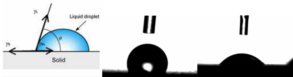
Figure 1.11. Contact angle ( \theta ) measured by goniometer. Middle image shows a water droplet on Teflon and the right image shows the same after conditioning of surface with surfactin.
