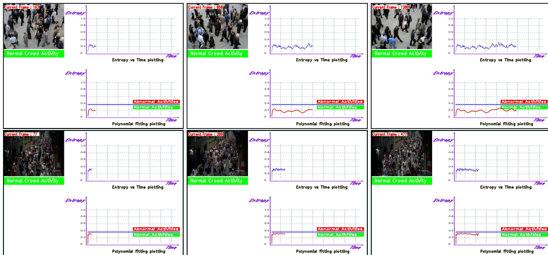
Figure 3.36: Qualitative results of normal behaviors detection. First and second rows concern normal activities of pedestrian walking and marathon running, respectively.
