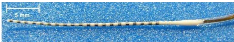
Figure 1.12. Macroscopic image of an intracochlear electrode implant embedded in a silicone matrix loaded with dexamethasone, adapted from 54
