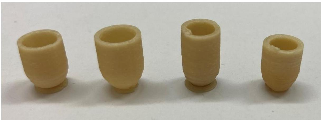
Figure 34 picture of several 3D printed capsules produced with DPE technology with the blend of aloe vera.
