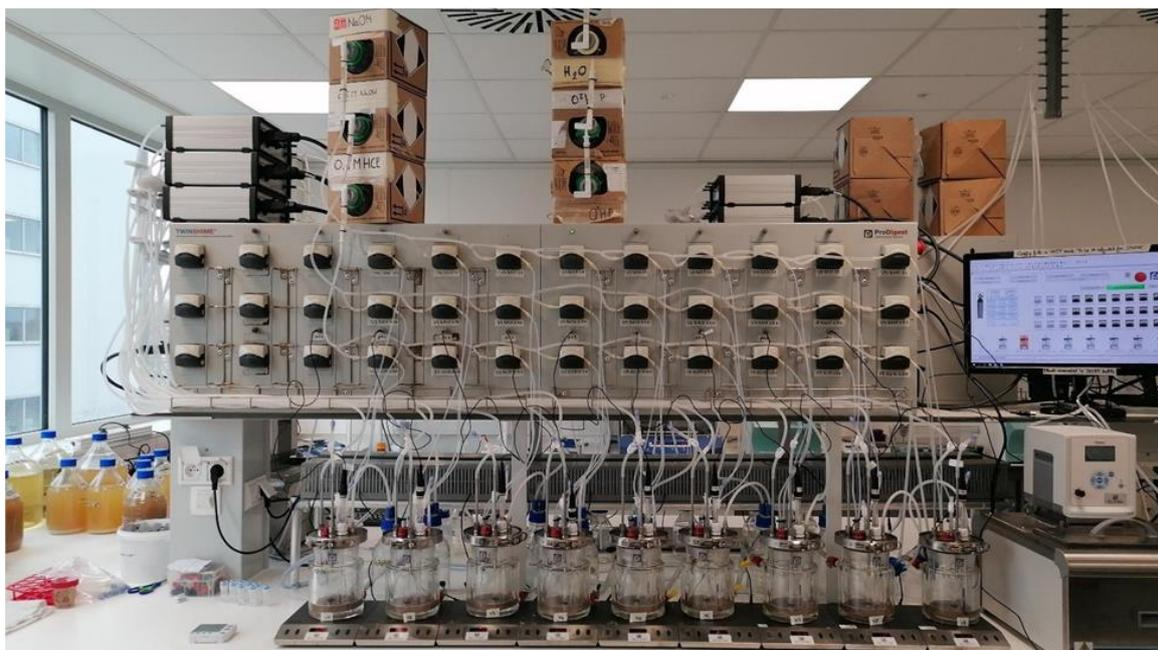
Figure 15 Fully automated computer-controlled semi-dynamic SHIME<sup>®</sup> model for colon-targeted drug delivery system testing. The system harbors nine separated bioreactors allowing to test 3 different conditions in biological triplicate at once. In each bioreactor the passage of the colon-targeted drug delivery system through the complete gastrointestinal tract is simulated by the sequential simulation of the stomach, small intestinal, and colonic phase.
