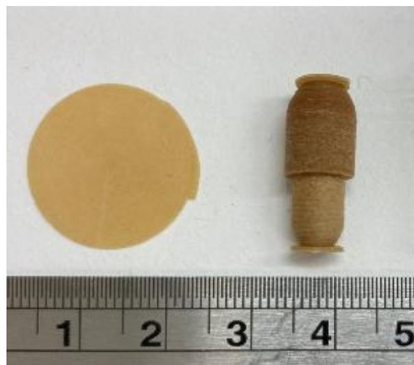
Figure 37 picture of 3D printed object produced with DPE technology using the blend of reishi extract.
