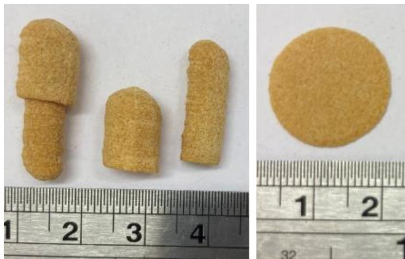
Figure 32 picture of 3D printed object produced with SLS technology with the blend of maltodextrin: a) capsule b) disc.
