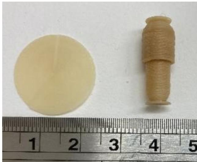
Figure 33 picture of 3D printed object produced with DPE technology with the blend of aloe vera.
