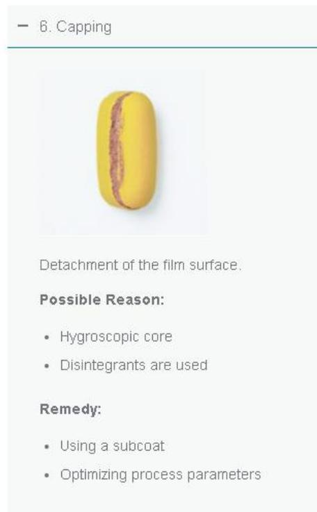
Figure 64: Capping phenomenon and its solutions.
