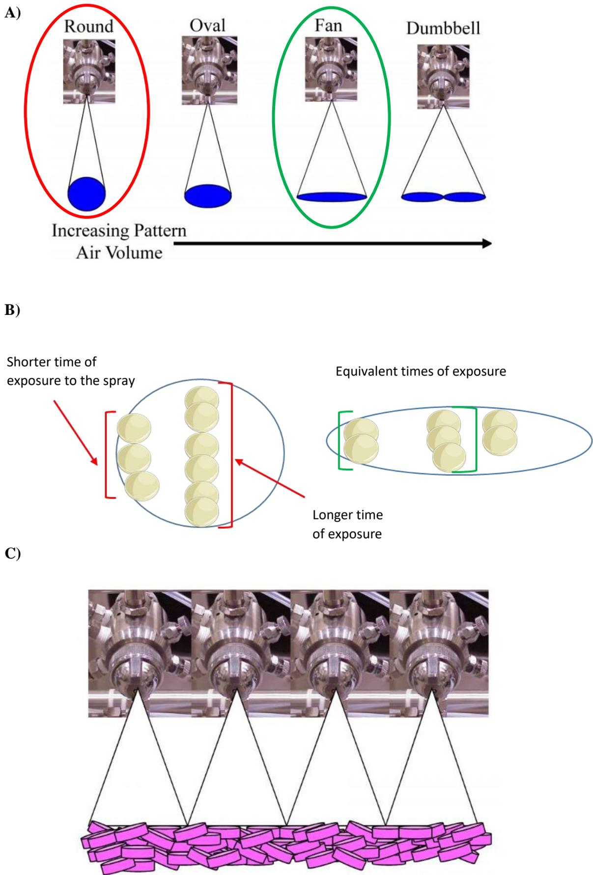
Figure 61: Uniform « curtain » of spray. Figures A) and C) reused from Freund Vector [36].
