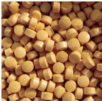
Figure 53: Tablets coated with Shellac:Inulin blends without ethylcellulose.
