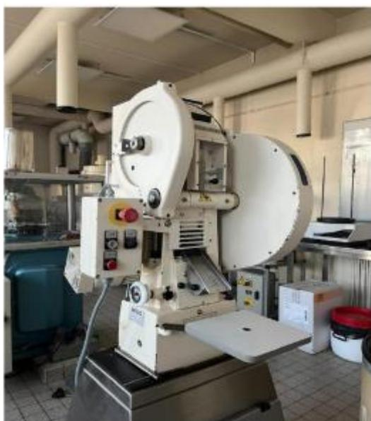
Figure 24: Single-punch tablet machine to get tablet cores (Korsch, EKO/DMS, Berlin, Germany).
