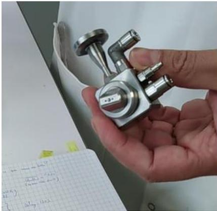
Figure 26: Spray nozzle and its body.
