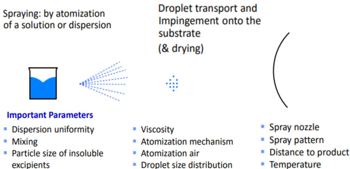
Figure 58: Film coating process with atomic layer deposition of polymer particles onto the substrate (tablet cores herein). Distance between nozzle and tablets bed as well as spray rate play a role for the film formation. Figure taken from Nyamweya et al. (2019, DOI: [10.13140/RG.2.2.34800.28164](https://doi.org/10.13140/RG.2.2.34800.28164)).
