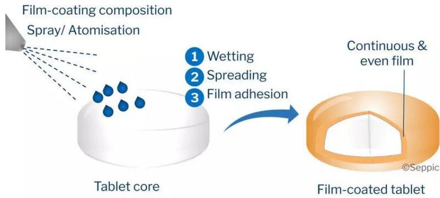
**Figure 29:** Coating process showing polymer particles coalescence around the tablet core. Figure taken from [SEPPIC](#) [151].
