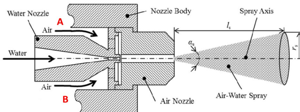
Figure 60: Schematic representation of the nozzle and its air flows. Shape air system can be seen on A and B zones. Figure reused from Herbst et al. (2016, <https://doi.org/10.1504/IJMMP.2016.079149>).
