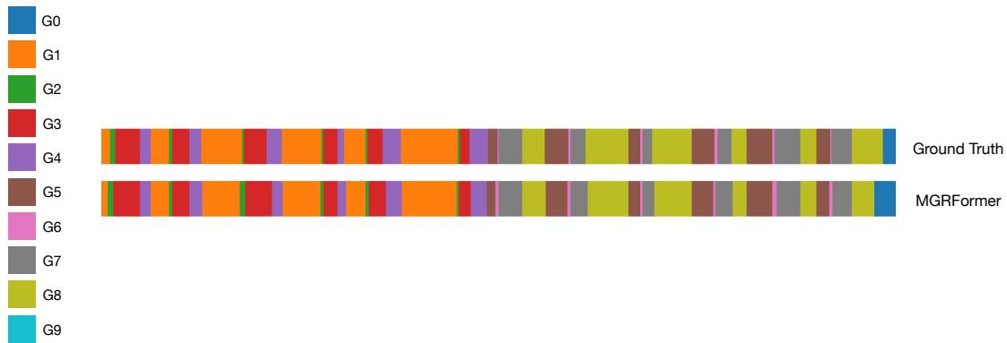
Figure 8.4: Color-coded illustration of surgical gesture recognition on the Peg Transfer dataset, comparing ground truth with MGRFormer _{k \rightarrow v} predictions, trained using surgical tools trajectory and I3D features.
