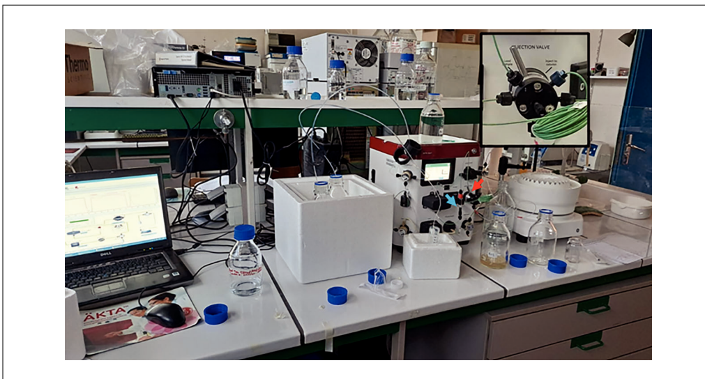
Figure 6 Overview of the protein purification and desalting process. The protein sample containing the POI is injected using an automated injection system (indicated by the red arrowhead) and shown in the inset above-right (sample loading position). The bottles for buffer A (lysis buffer) and buffer B (elution buffer) are in the central polystyrene box. Fractions are collected using an automatic collector at the right of the picture. The process is monitored by measuring absorbance at a specific wavelength of 280 nm thanks to a computer at the left. The device is shown in its desalting configuration: the HiTrap Desalting is indicated by the blue arrowhead.
