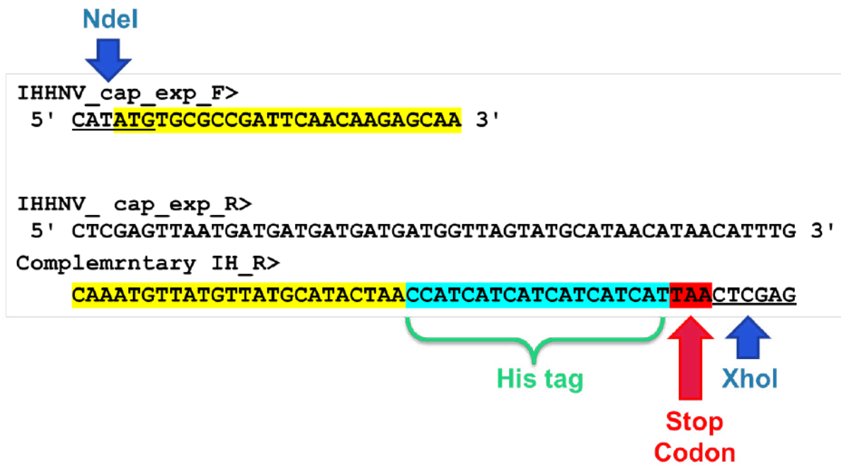
Figure 4.1: IHHNV capsid gene (ORF3) specific primers. Top: forward primer with NdeI cutting site. Bottom: reverse primer with Histidine-tag, stop codon and XhoI cutting site.
