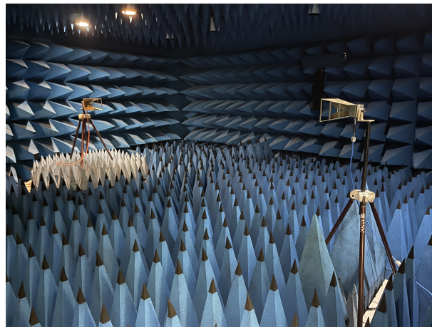
Figure 5.27: Radiation pattern measurements in an RF Anechoic chamber
