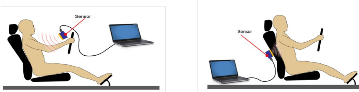
Figure 2.10: (a) The radar is 0.5 m in front of the person, (b) The radar is installed behind the seat [99]
