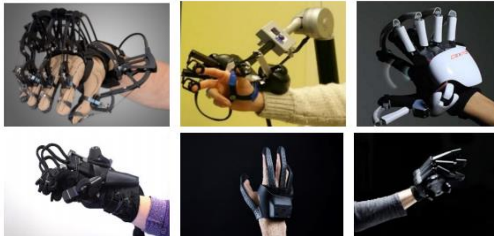
Figure 11. A few examples of commercial haptic feedback gloves. In order: CyberGrasp, H-glove, Dexmo, HaptX, Plexus, and VRgluv [58].
