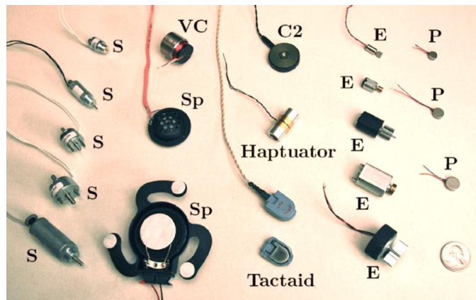
Figure 12. Sample actuators for vibrotactile displays. S: Five solenoids of varying sizes. VC: A commercial voice coil without bearings. Sp: Two audio speakers. C2: A C2 factor from EAI. Haptuator: A Haptuator from Tactile Labs, Inc. Tactaid: One complete Tactaid from AEC and one opened to show the suspension inside. E: Five shafted/cylindrical eccentric rotating mass motors. P: Three shaftless/pancake eccentric rotating mass motors. A U.S. quarter appears at bottom right for scale [83]
