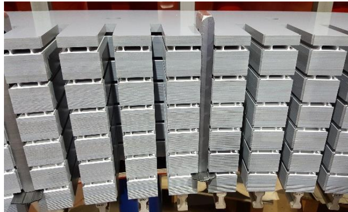
Figure I.3. Stator core of the Hydro generator La Coche - G5 (237,8 MW) during the assembly step (Image from EDF).
