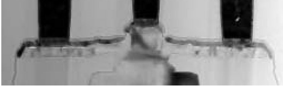
Figure I.9 | TEM cross section of the Elevated Extrinsic Base - Selective Epitaxial growth (EBL-SEG) HBT presented by Manger et al. [40].
