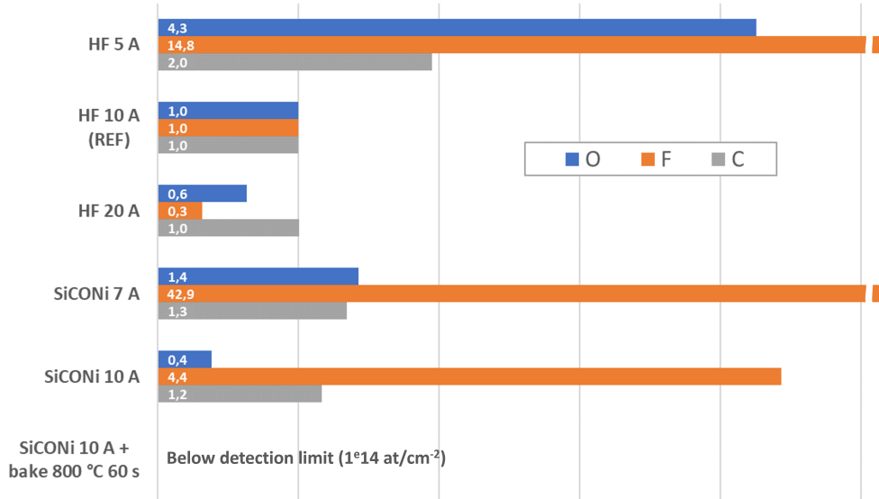
Figure II.28 | Relative total dose of oxygen, fluorine and carbon at the interface. Integration performed on the curves of figure II.27 over the same span. HF 10 A is taken as reference.
