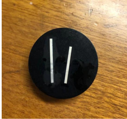
Figure II-4. Samples prepared for indentation test.
