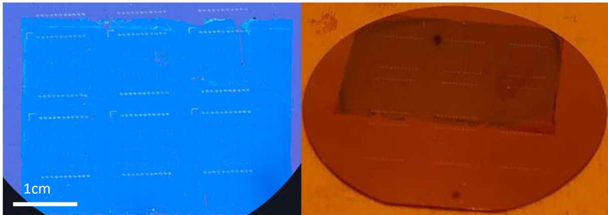
Figure 24 Optical photography of SS07 after deposition of the 3 MLs of MoS 2
