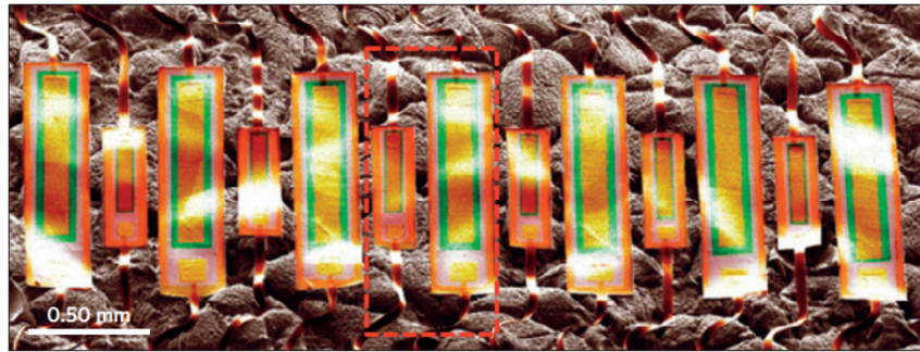
Figure 1.16: Thin, compliant modulus sensor (CMS) based on nanoribbons of PZT in arrays of mechanical actuators and sensors [35].
