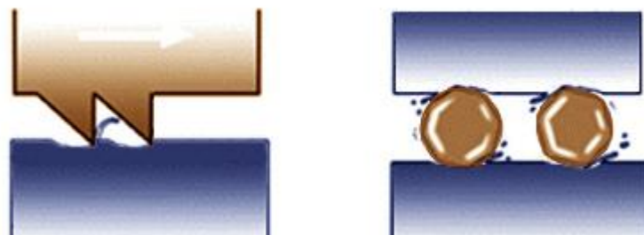
Figure 2: Abrasive wear schematic
