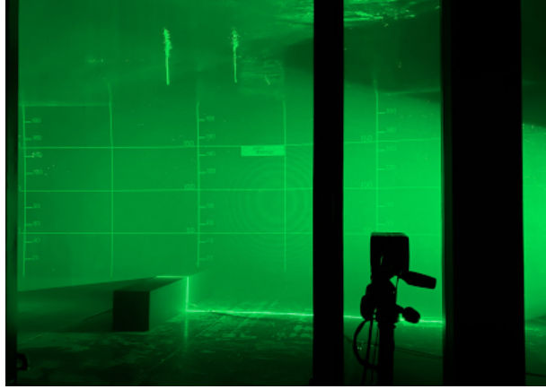
FIGURE 2.3 – PIV setup with the camera in foreground and the laser sheet illuminating the square cylinder. The resistive wave probes are passing through the free-surface where a wave-trough is visible on top of the cylinder.
