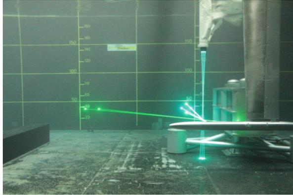
Figure 4.16 – 2C- and 3C-LDV measurement between the bathymetry obstacle and the ducted 2-VATT model in the Ifremer's tank.
