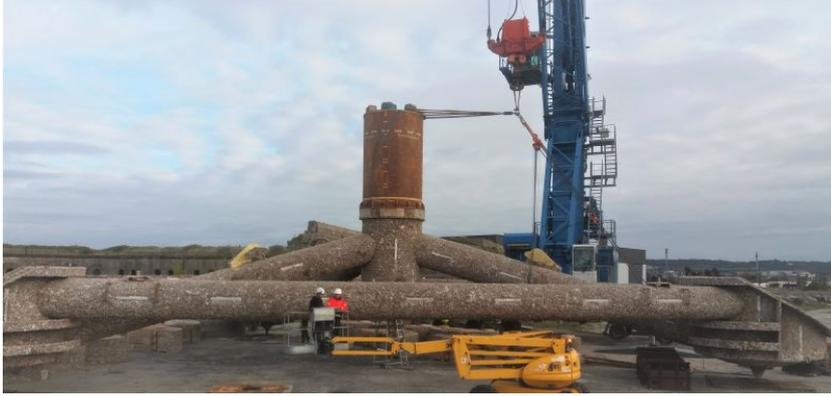
Figure 2.17 – Setup used to calibrate the strain of the gauges with regard to the horizontal load applied at the top of the base mast.
