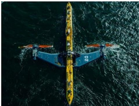
(c) O2 turbine at the Fall of Warness test site
