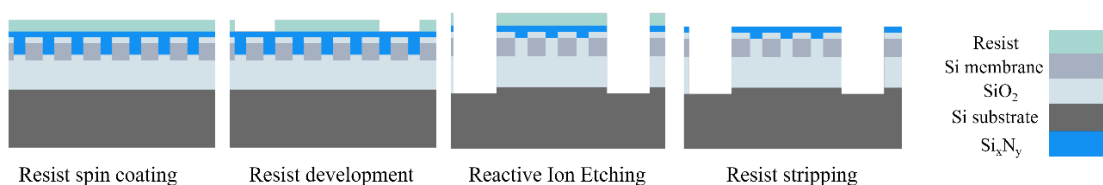
Figure 3-26: Cavities opening process steps.
