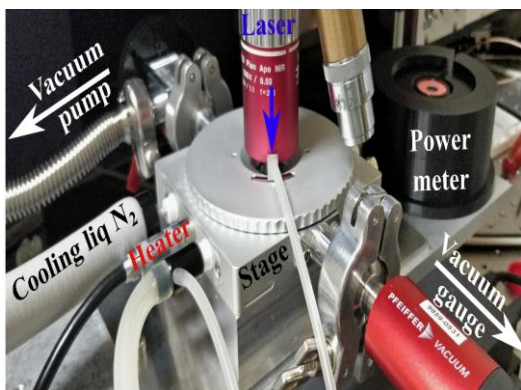
Fig 3.9 Heating/ cooling stage from Linkam – connections showing vacuum gauge, liquid N2 cooling and heater attachment. A Si-photo diode power meter from Thorlabs
