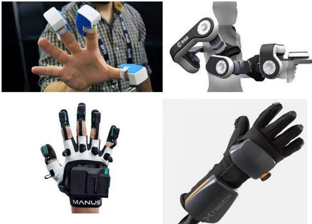
Figure 1.13: Examples of kinesthetic feedback devices. Starting from the top: Fingertip-mounted devices [51], Space Exoskeleton Controller (SPOC) [52]. On the bottom: Manus Quantum Meta-glove [53] and (d) HaptX glove G1 [54].
