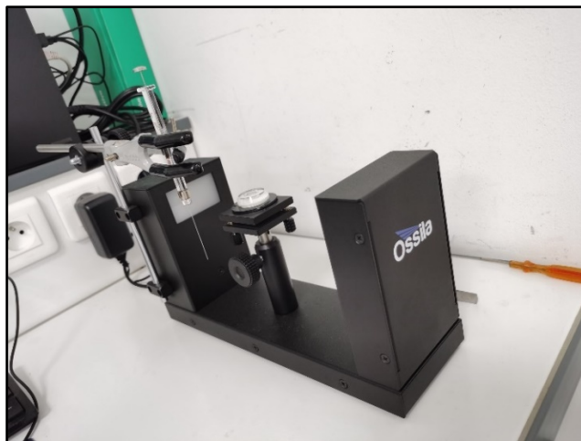
Figure 2.6. Ossila L2004A1 instrument used for the determination of the water contact angles.
