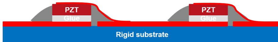
Figure 4.2: Cross section of the first steps of fabrication.
