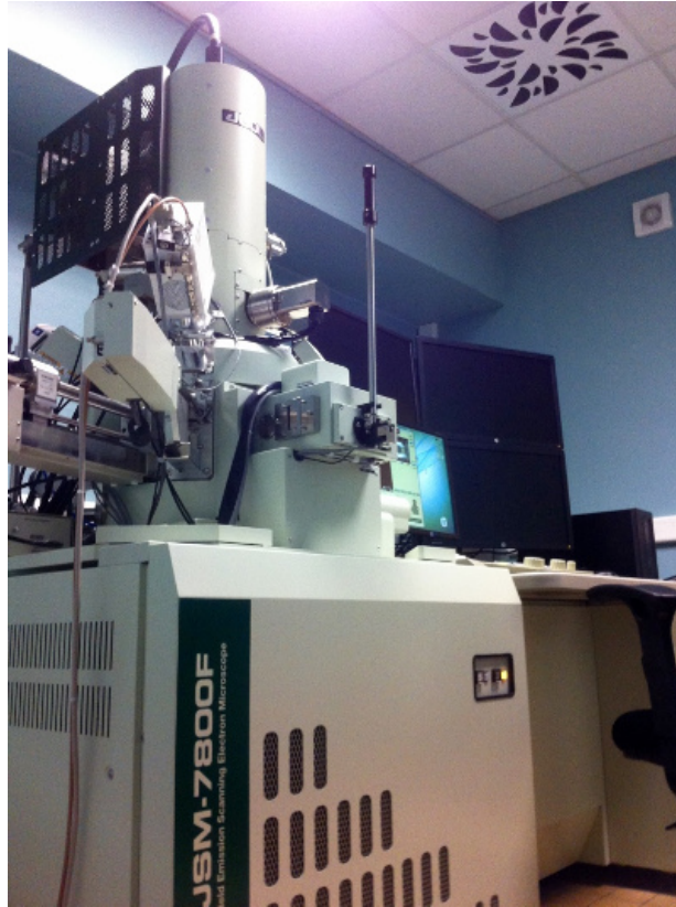
Figure 2.1. Photo of JEOL JSM-7800F field-emission scanning electron microscope.
