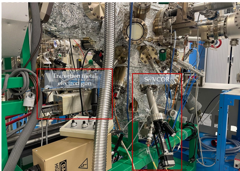
Figure 2.3: TMDC reactor specificities
