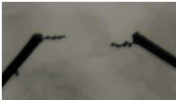
Figure 4.7: Dendritic growth after 40 min of electropolymerization for a monomer concentration of 2.5 mM, under the set of specified experimental conditions, as detailed in the text.
