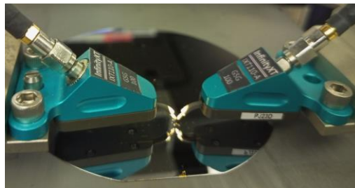
Fig. 3.2: DC measurement with GSG probes.
