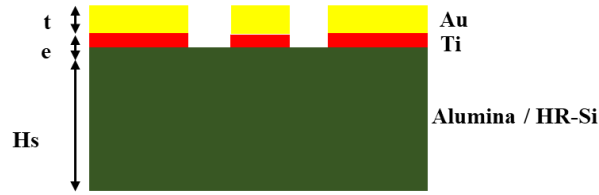
Fig. 2.2: Cross-section of CPW line.
