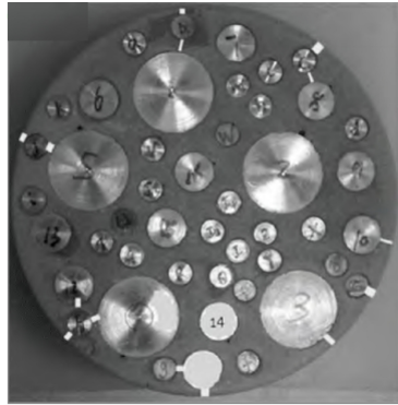
(a) The test sample and the crack distribution (white part) (b) Relative humidity curve with drying time at 0 mm, 10 mm and 20 mm away from the surface
