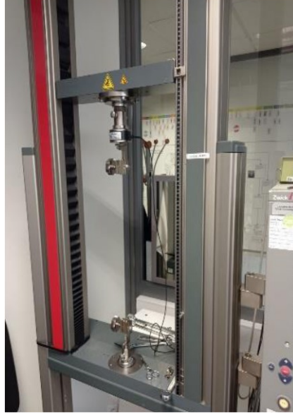
FIGURE 3.8: Tensile testing device used for inlay yarn characterisation [113].
