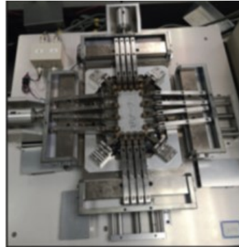
FIGURE 2.13: Biaxial test on cut-strip samples of medical compression stockings [44].
