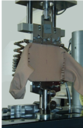
FIGURE 2.10: Tensile test on cylindrical samples of medical compression stockings [30].
