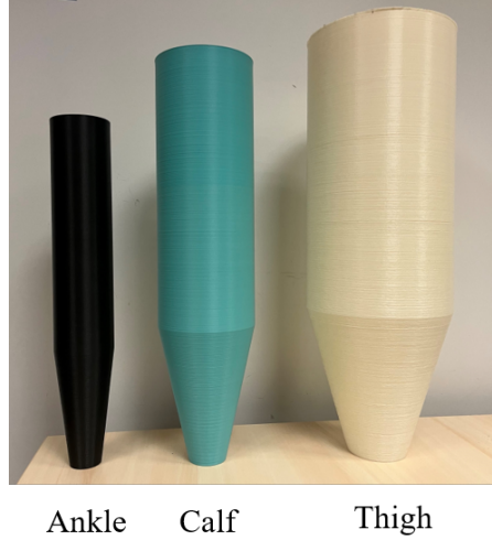
FIGURE 3.31: Three dimensional printed rigid leg models corresponding to the maximal leg perimeters ( P_{\text{leg,max}} ) of the three compression zones
