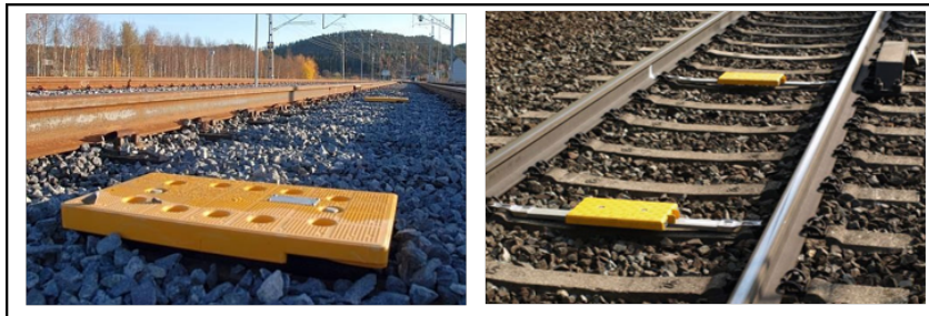
Figure 2.14: Physical Balises (PB) and Balise Groupe (BG)
