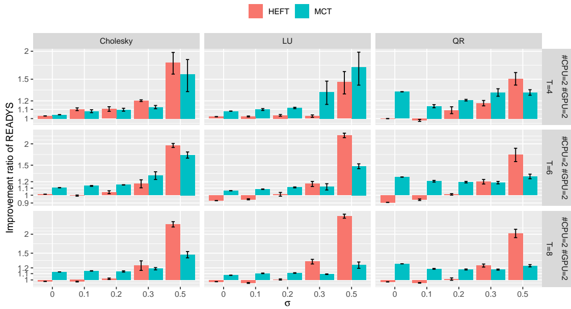
Figure 4.2 – Makespan improvement over HEFT and MCT according to T \in \{2, 4, 8\} (rows), the noise level \sigma , and for each of the 3 tasks we consider (3 columns), when the computing platform is made of 2 CPUs and 2 GPUs. The larger the bars above 1, the better READYS performs w.r.t. to competitors.
