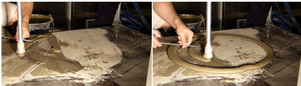
Figure A.5: The first layer of the cylindrical shape designed for manual calibration of the printing system parameters based on the measurement of layer widths.
