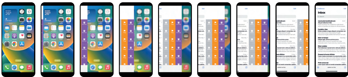
Figure 5.7 – Adapted ‘Forward and backward’ animation of an email application opening, with the application sliding in from the right side, revealing the swhidgets to the right of the usual application view before reaching its end position.
