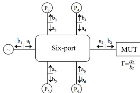
Figure 5.1 Block diagram of six-port reflectometer [95].
