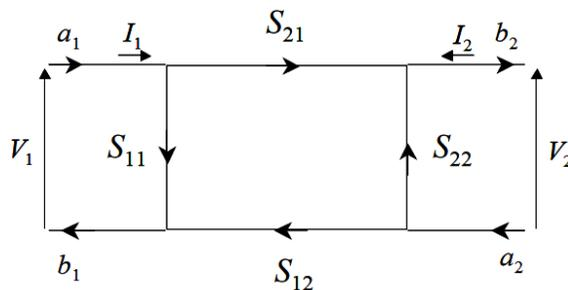
Figure 3.2 Graph illustrating a quadrupole circuit [95].
