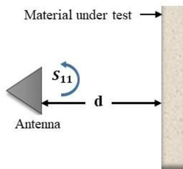
Figure 3.5 Principle of monostatic free-space measurement [17].
