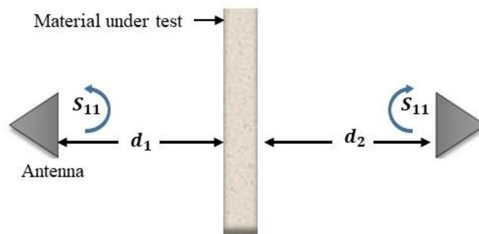
Figure 3.4 Principle of bi-static free-space measurement [17].
