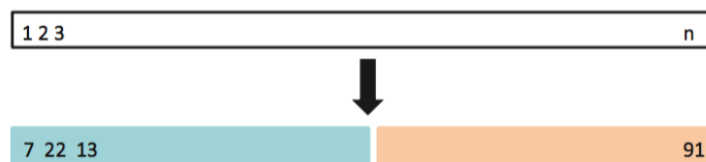
Figure 2.6: Cross-validation: The naive cross-validation splits the dataset into a 50/50 division as the training data and the test data. [Adapted from 77]
