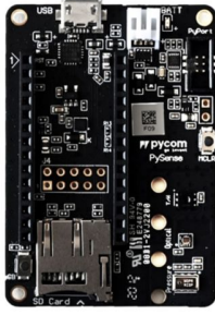
Figure 3.4: External shield - Pysense
